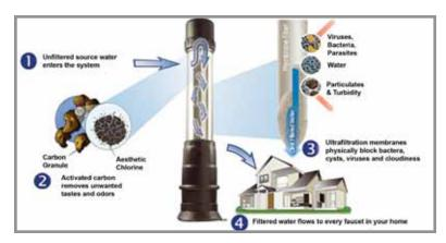
The System consistently provides clean, filtered water for all of your cleaning, cooking, washing and drinking needs; while automatically flushing unwanted contaminants and particles down the drain.
